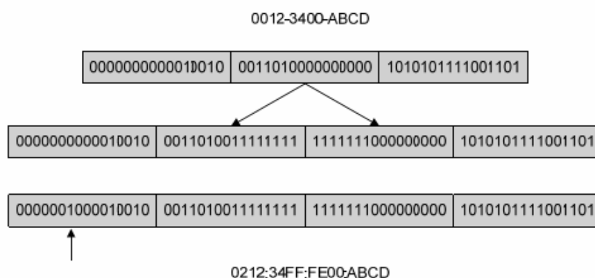
Figure 1-2 conversion process from MAC address to EUI-64 format interface identifier
